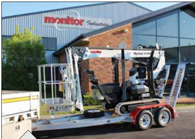
This spider's light weight and compact stowed size allows easy transportation. This package, including the trailer, weighs approx. 2t.
