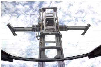
FOPS Compliant Top Glass for optimal Optimal Driver Visibility (Standard)
