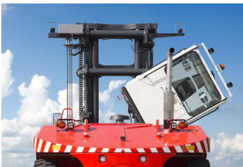
Tilting Cab for Easy Access to Drive Train & Hydraulics
