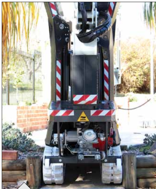
The light-weight basket is simple to remove in less than one minute, allowing very narrow access and reducing the stowed length to only 3.69m
