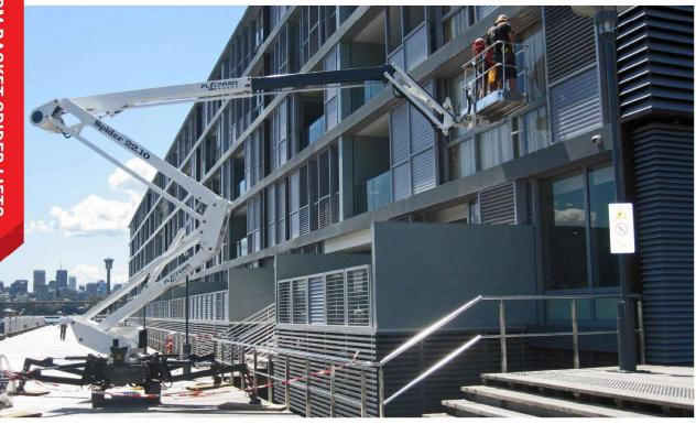
Excellent up-and-over reach with modern double-knuckle technology, and adjustable fly-jib for extra manoeuvrability.
