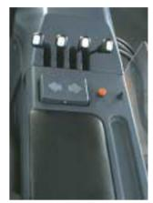
The efficient layout of the operating control levers and direction switch are another example of Toyota practicality. Here minimal operator effort is needed to safely and productively use the controls.
