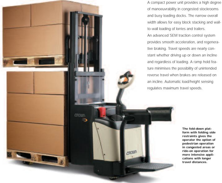
The fold-down platform with folding side restraints gives the operator the option of pedestrian operation in congested areas or ride-on operation for more intensive applications with longer travel distances.
